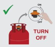
Make sure the regulator knob on the cylinder is turned off
